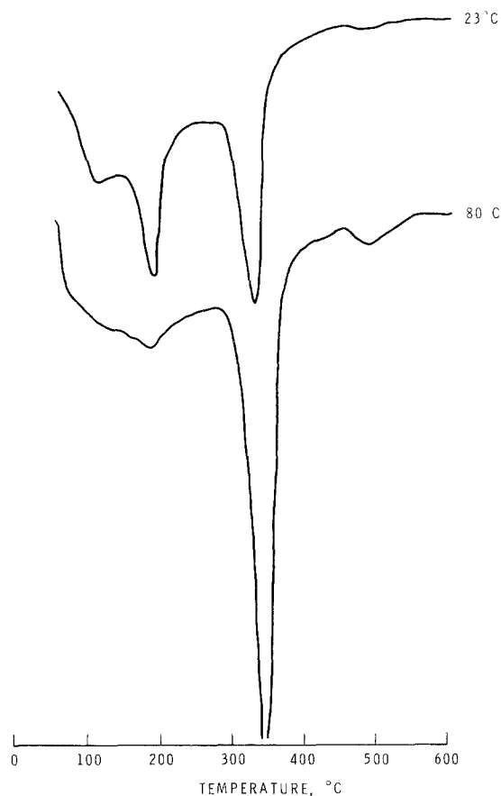
Figure 1 DSC curves for \text{C}_4\text{AF} hydrated for 2 days at a W/S ratio of 0.13.
